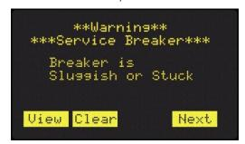
initiates a breaker trip, it measure the time between triggering the actuator and when each pole interrupts the current. If this time is greater then the setting, the Sluggish Breaker alarm is set. If the Sluggish Breaker alarm is set, that is an indication that the breaker mechanism is in need of service. The internal logic of the electronic trip unit performs self-diagnostics and will generate and alarm if self-testing fails.
